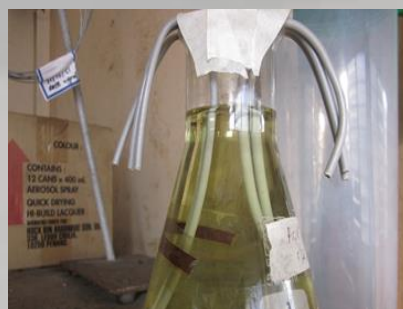
50% Acid hydrochloric test on PVC penetration to wires
