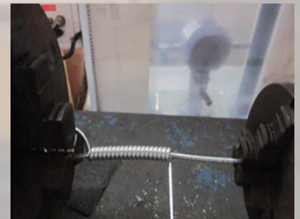
Galvanized wire wrapping test on its own diameter (mandrel 1XD) more stringent than BS specification requirement.
